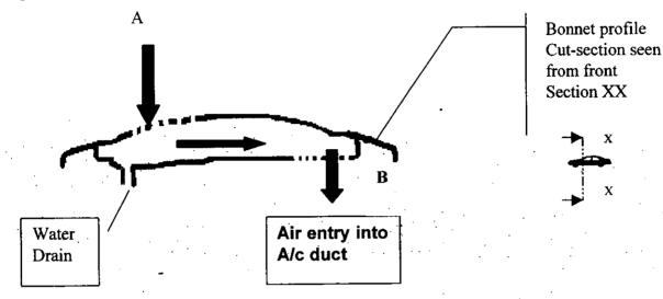
Direction of Airflow to air-conditioning system through fins on bonnet top. This is applicable for RHD vehicles.
